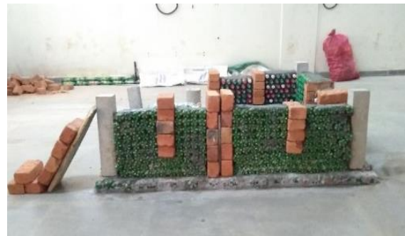
Figure 21 Concrete prisms placed in four corners
