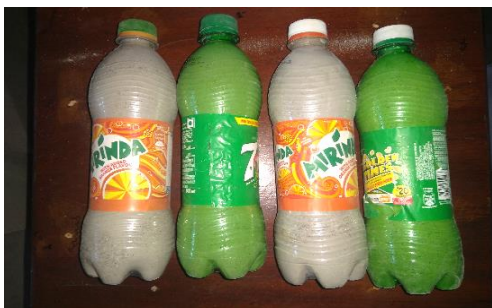
Figure 5 Bottles filled with demolished concrete waste (Sample 1)
