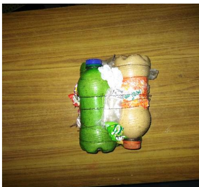
Figure 2 Bottles filled with saw dust
