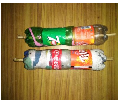
Figure 10 Bottle units made using plastic wrappers as the filler material and bamboo sticks as reinforcement
