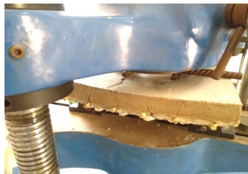
Figure 13 Bottle panel at its breaking point when loaded in UTM
