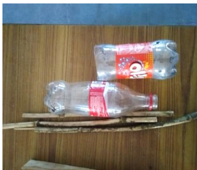
Figure 9 Two bottles and one bamboo stick for a single bottle unit
