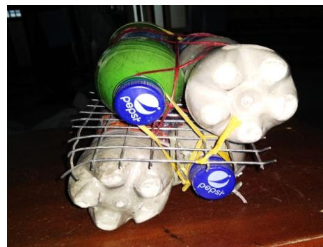
Figure 7 Chicken wire mesh placed in between the bottles (Sample 2)
