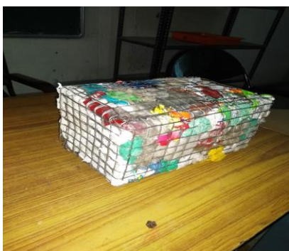
Figure 3 Block placed in chicken wire mesh cage
