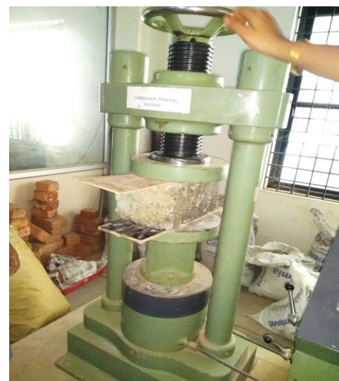
Figure 15 Concrete block loaded in CTM
