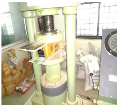
Figure 4 Block loaded in CTM
